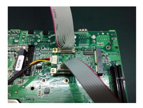
**Step 5** Connect the power cable to the 4PIN power connector
