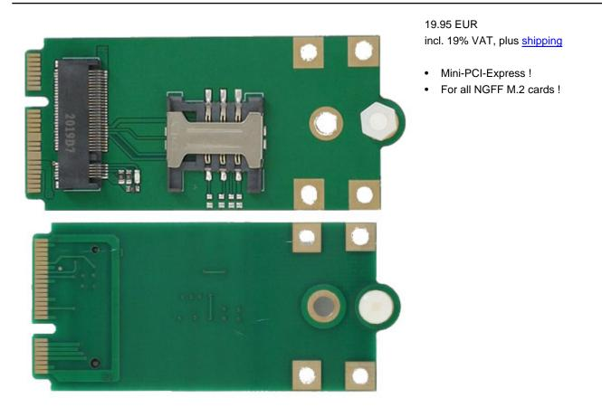
This adapter enables you to use a NGFF (M.2) modem card in a Mini-PCI Express slot. The adapter works in all systems with Mini PCI-E slot (eg. EmbeddedPC, CarPC, MiniPC, Laptop, TabletPC, Android, etc..)
